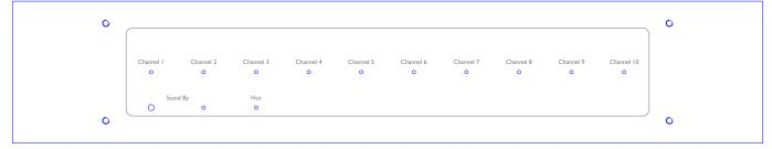
The C50 contains ten identical channels of audio amplification. Unless otherwise stated, this section refers to one channel only.
